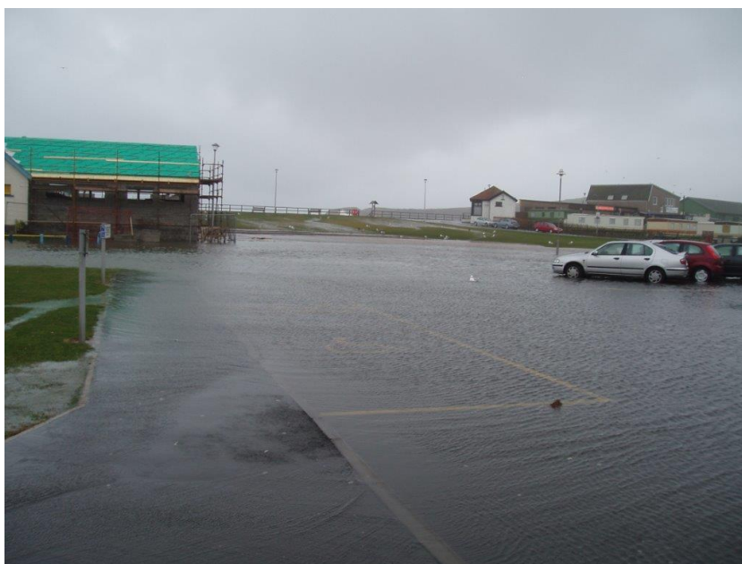
Flooding of car park behind swimming pool due to overland flow from overtopping of Cowie promenade. Photograph supplied by Aberdeenshire Council.
